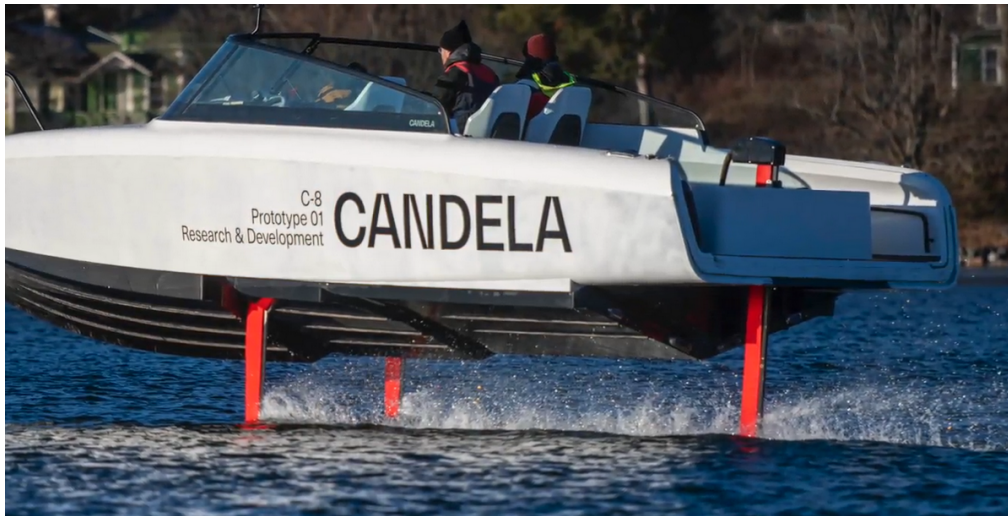
Figure 2.2: Image of a Candela C-8 equipped with fully submerged hydrofoils. [2]
