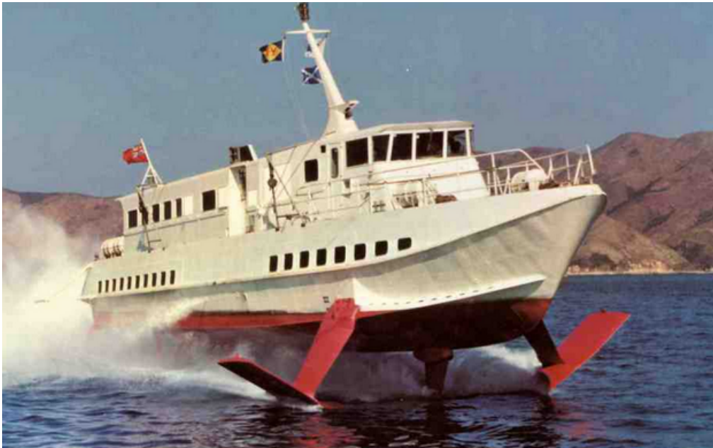
Figure 2.1: Image of a boat using U-shaped surface-piercing hydrofoiling. [1]
