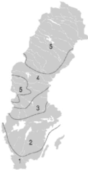
Figure 5. Climate zones used for the structural design of roads according to TRVK Väg (Trafikverket, 2011).
