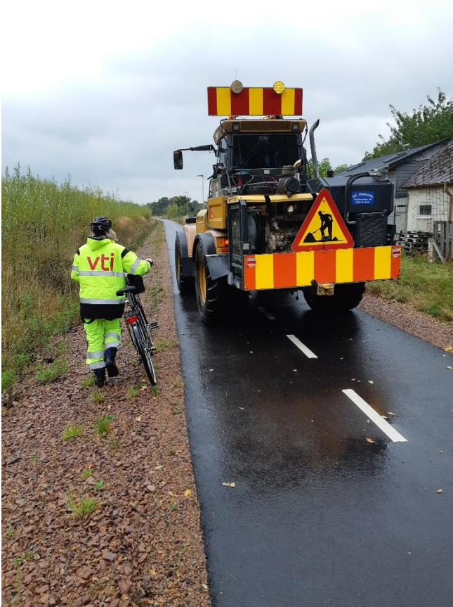
Figure 7. Heavy maintenance vehicle transiting a cycle path in Skåne, Sweden. Note the vehicle's wheel span width in relation to the width of the cycle path, and how close to the edge that the wheels are.
