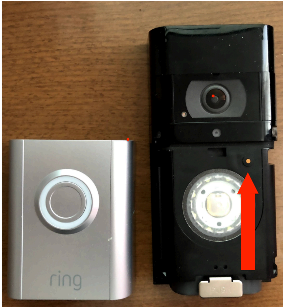
Figure 3.2: Ring Doorbell 3 Plus setup mode button
