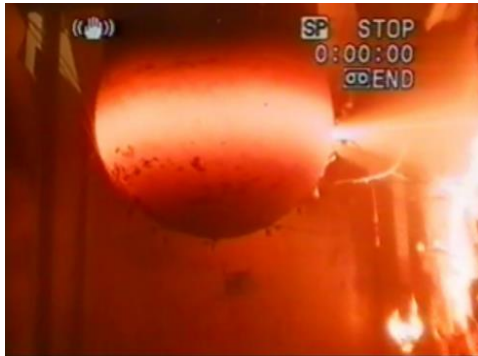
Figure 3.2. Rupture phenomenon in FOREVER Test [24]
