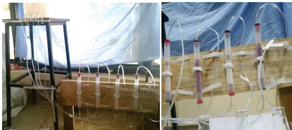
Figure 36. Mini-scale column to evaluate efficiency of magnesite, bauxite, gypsum, and BGM (1:1:2).
