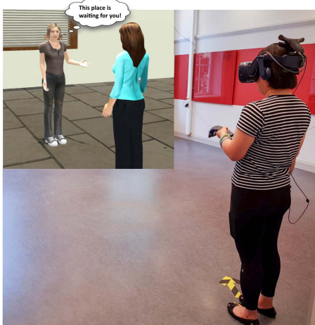
Figure 2: A participant immersed in the VE during the user study, standing at the prescribed starting position and orientation to begin each trial. Free walking in the room is enabled by the wireless adapter mounted on top of the HTC VIVE Pro headset, and connected to a battery pack.
