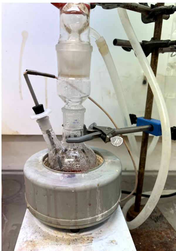
Figure A.0.5: Image showing the hydrolysis setup
