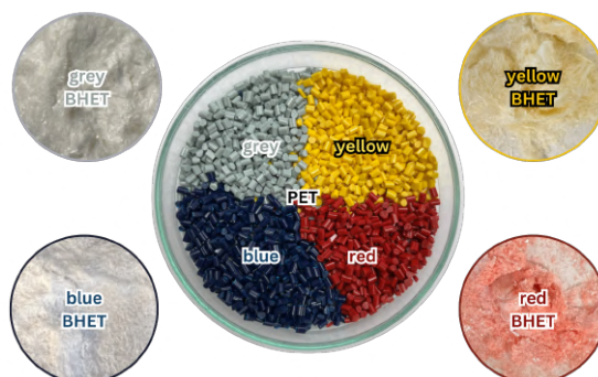
Figure 4.1.1: Overall Result of the Glycolysis
