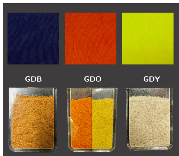
Figure 1.2.1: Dispersed dye fabrics compared to their depolymerised monomers[6]
