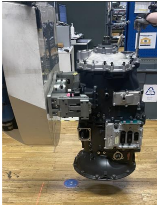
Figure 8: Assembly of the planetary gear, control unit and the back cover. (courtesy: Scania)
