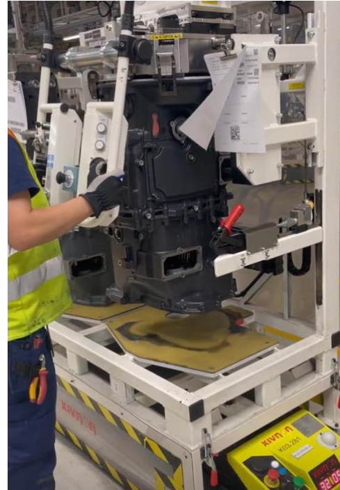
Figure 4: An operator placing the gearbox on an AVG (courtesy: Scania).
