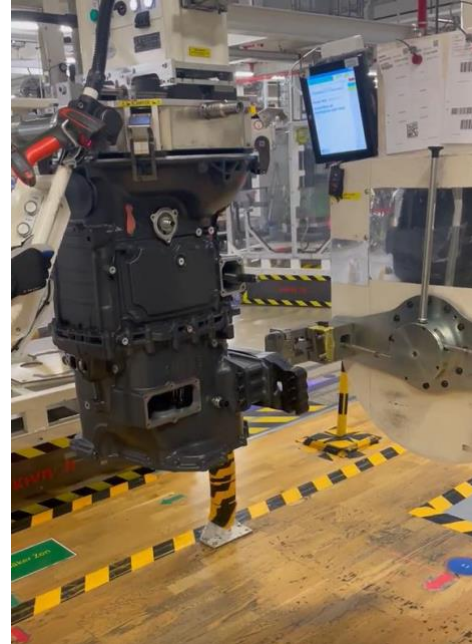
Figure 6: An Operator is lifting the gearbox from the AVG and mounting it on a carrier in the main line (courtesy: Scania).
