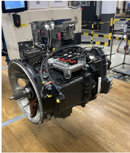
Figure 10: The gearbox is nearing the end of the main line. (courtesy: Scania)
