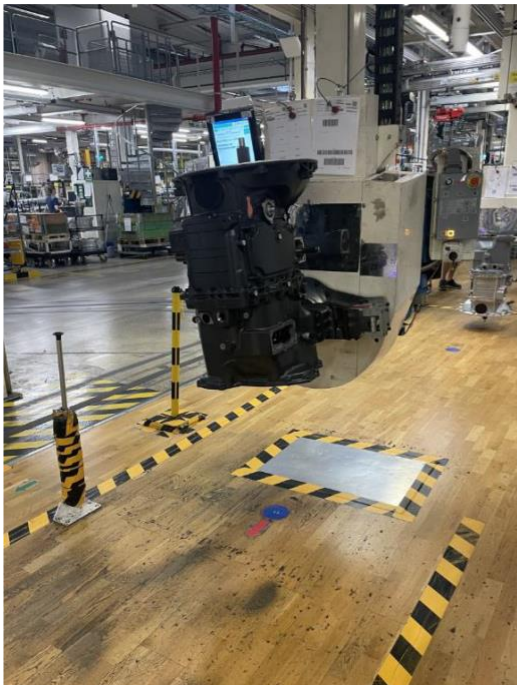
Figure 7: The gearbox on its way to the first assembly station. (courtesy: Scania)
