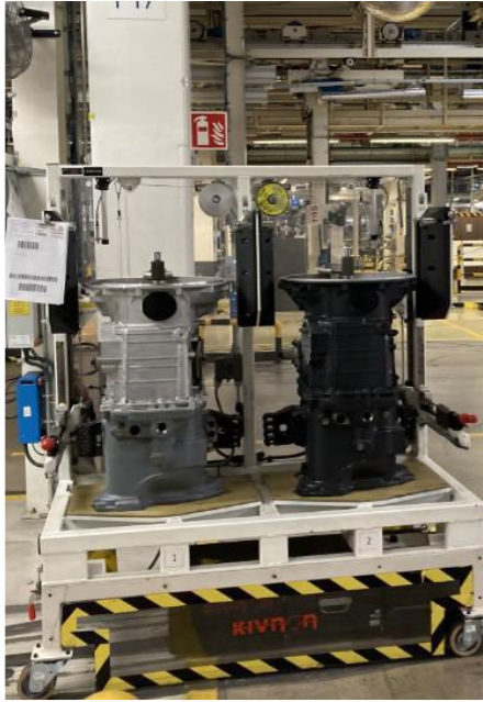
Figure 5: The AVG transporting the gearbox to the main line (courtesy: Scania).
