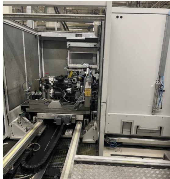
Figure 12: The gearbox is going through the test run using the same test program as the new gearboxes. (courtesy: Scania).
