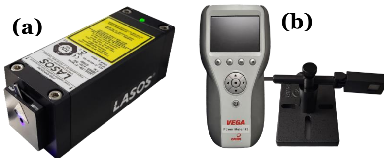
Figure 3.1: Devices used for micro optics testing: (a) CW LD Lasos LDM-XT, with a max average output power of 120 mW, and center wavelength at 405 nm, (b) power meter Ophir Vega color laser power & energy meter, and 300 mW silicon photodiode Ophir PD300-UV.
