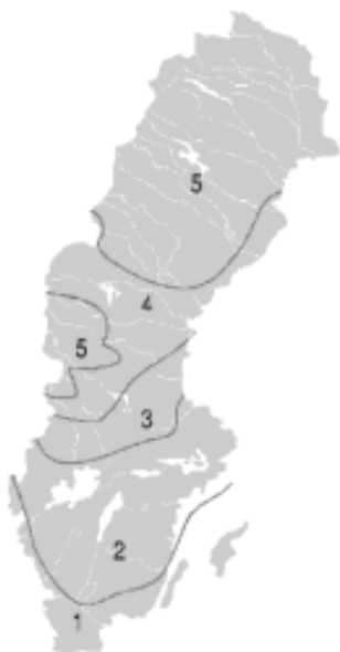
Figure 7. Climate zones used for the structural design of roads, according to TRVK Väg (TRV, 2011a).
