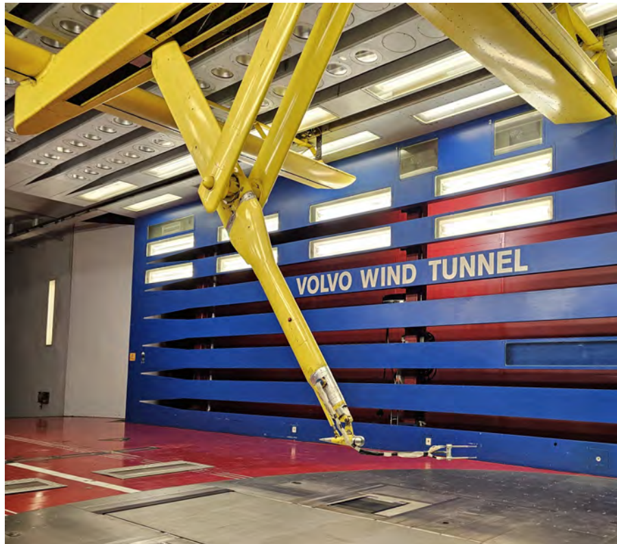
Figure 4.3: Dual probe measurement system on the traverse used for static pressure measurements. The probe is in its "standard" orientation in this image. Image taken by the author, published with permission of Volvo Cars.
