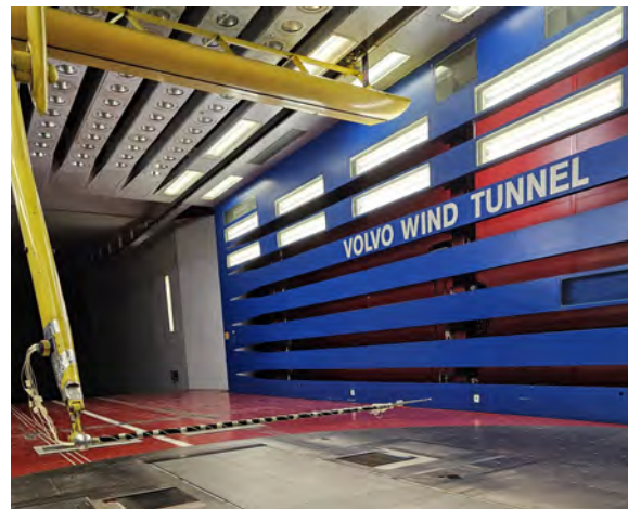
Figure 4.5: Omniprobe mounted on long pole away from the traverse, for testing the influence of the traverses proximity to the measurement device. Image taken by the author, published with permission of Volvo Cars.
