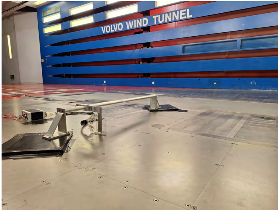
Figure 4.7: Boundary layer rake set up, the rake can be moved along the beam to specific locations and locked in place. Image taken by the author, published with permission of Volvo Cars.
