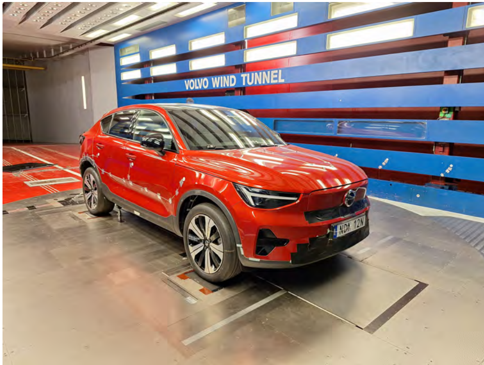
Figure 4.9: Picture of the Volvo C40 being tested with pressure patches mounted onto the body of the vehicle. Image taken by the author, published with permission of Volvo Cars.
