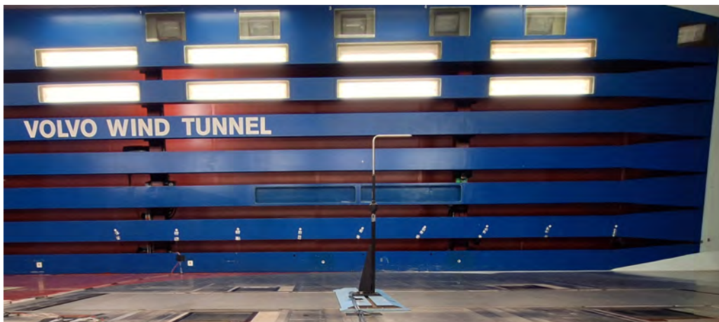
Figure 4.11: Picture of the Pitot tube mounted in the wind tunnel for wind speed calibration. In the background can be seen the pressure patches mounted on the wall of the test section. Image taken by the author, published with permission of Volvo Cars.
