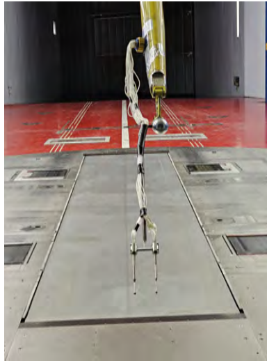
Figure 4.4: Dual probe measurement system on the traverse used for static pressure measurements. The probe is rotated 90° from its "standard" orientation in this image. Image taken by the author, published with permission of Volvo Cars.
