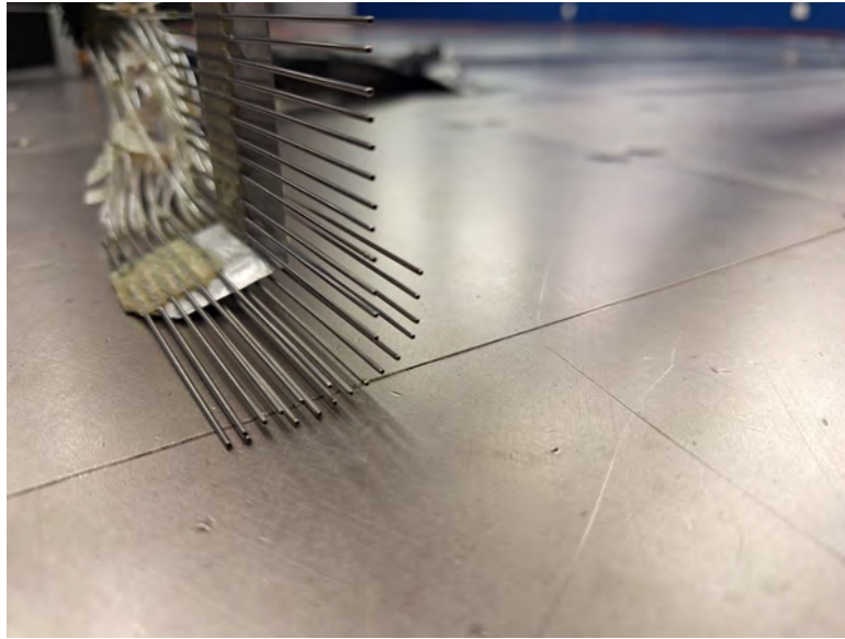
Figure 4.6: Close up shot of the boundary layer rake employed for the experiments. Image taken by the author, published with permission of Volvo Cars.
