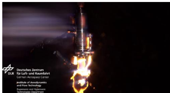
Figure 44: Whole thruster at 0 ° demise behaviour in DLR's PWT test [40].
