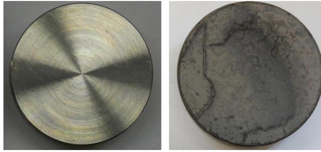
Figure 27: Titanium alloy Ti6Al4V – Photographs before and after testing in L2K DLR PWT [37].
