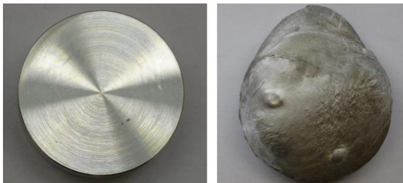
Figure 25: Aluminium alloy 7075 – Photographs before and after testing in DLR's PWT [37].
