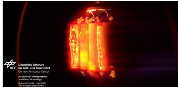
Figure 39: Battery Module demise behaviour in DLR's static PWT test [44].
