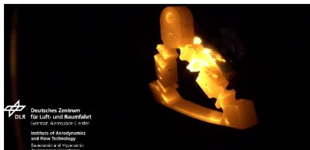
Figure 48: Holes bipod demise behaviour in DLR's PWT test [39].
