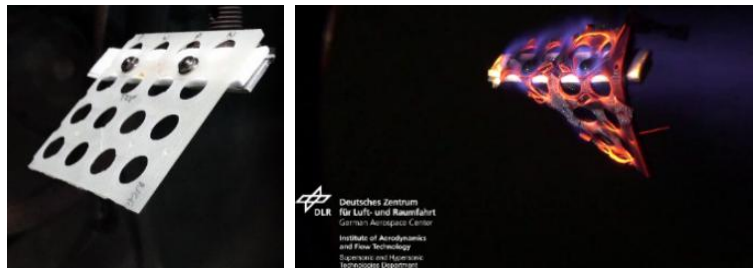
Figure 35: GFRP sheet of battery module demise behaviour in stagnation configuration in DLR's PWT facilities [44].
