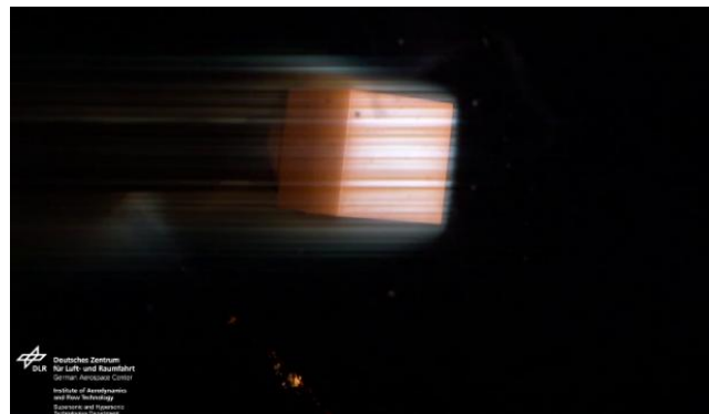
Figure 32: Tungsten cube demise behaviour in PWT test [41].
