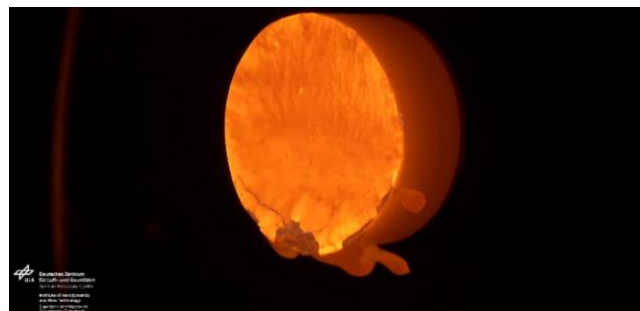
Figure 30: Inconel 718 demise behaviour and oxide layer collapsing in PWT test [40].
