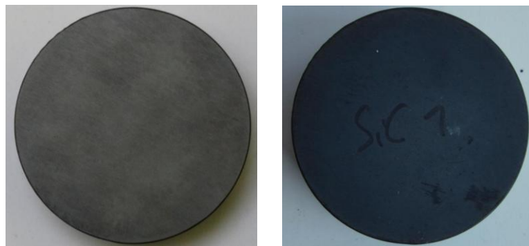
Figure 20: Silicon carbide SSiC ultra-pure – Photographs before and after testing in L3K PWT test [37].
