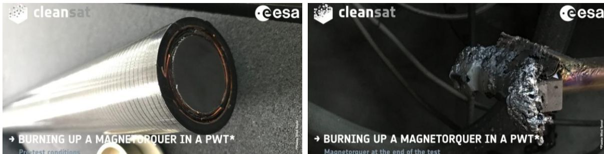
Figure 9: MTQ burning up in a PWT before and after the test [25].
