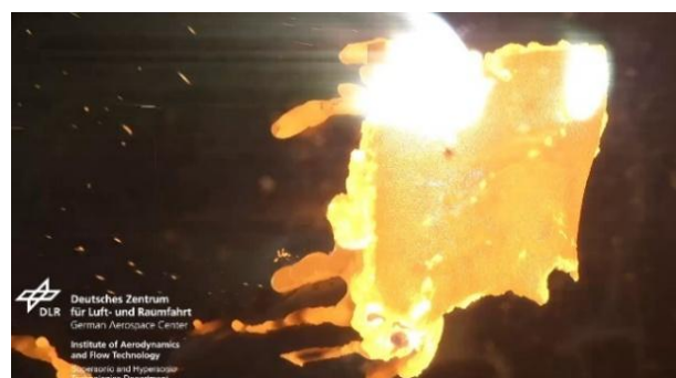
Figure 31: Molybdenum and Titanium screws demise behaviour in PWT test [41].
