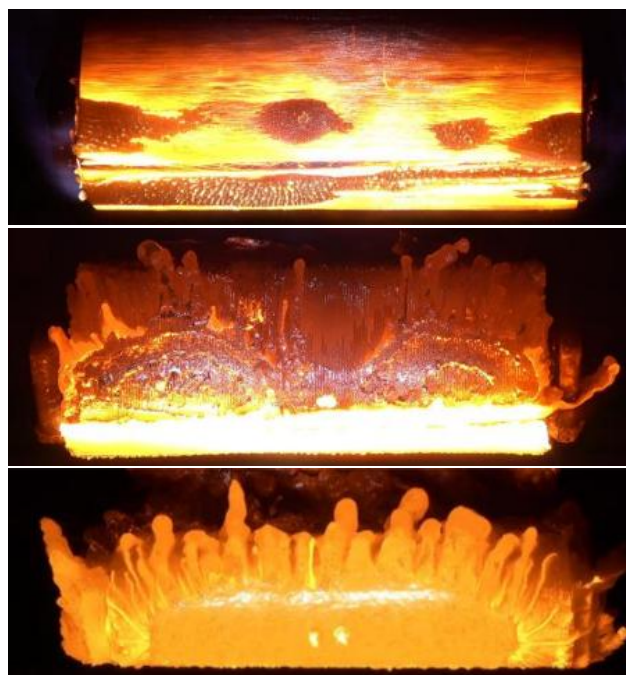
Figure 46: MTQ demise behaviour in PWT test, showing the CFRP burn through, layer-by-layer Coil removal and core melt from up to down [55].
