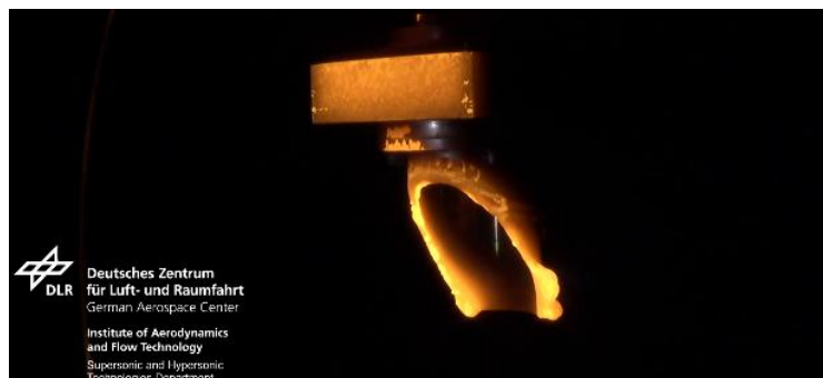
Figure 47: Star tracker demise behaviour in DLR's static PWT test and high-flux conditions [44].
