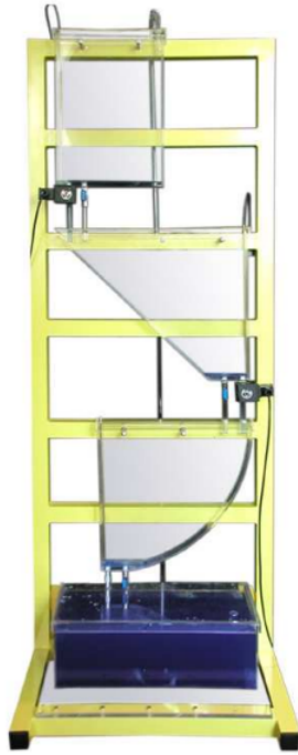
Figure 3.4: Three-tank system: valves \gamma_1, \gamma_2, \gamma_3 are control inputs; pump inflow q is a measured disturbance. States are levels h_1, h_2, h_3 ; constraints \mathcal{X}, \mathcal{U} are safety-critical.
