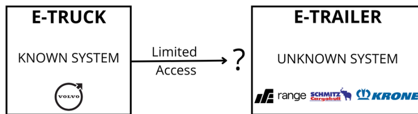
Figure 1.2: System overview, the e-truck (known, controllable) interfaces with an e-trailer treated as an unknown subsystem; only limited signals are available across the truck–trailer link, motivating online identification and safety-aware control.
