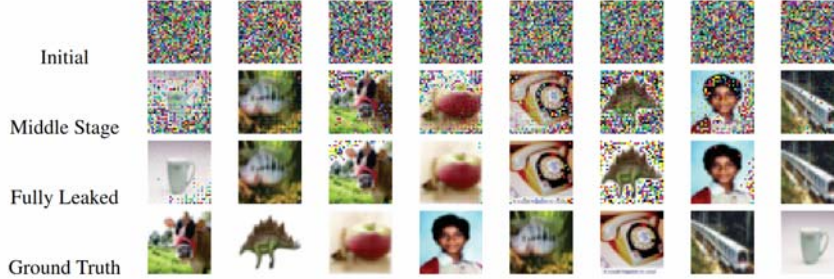
Figure 3.2: DLG reconstruction of a batch of 8 samples (extracted from [8]). The dummy inputs are randomly initialized, and are fully leaked after 2711 iterations (up to a permutation). The model used was a ResNet-20.
