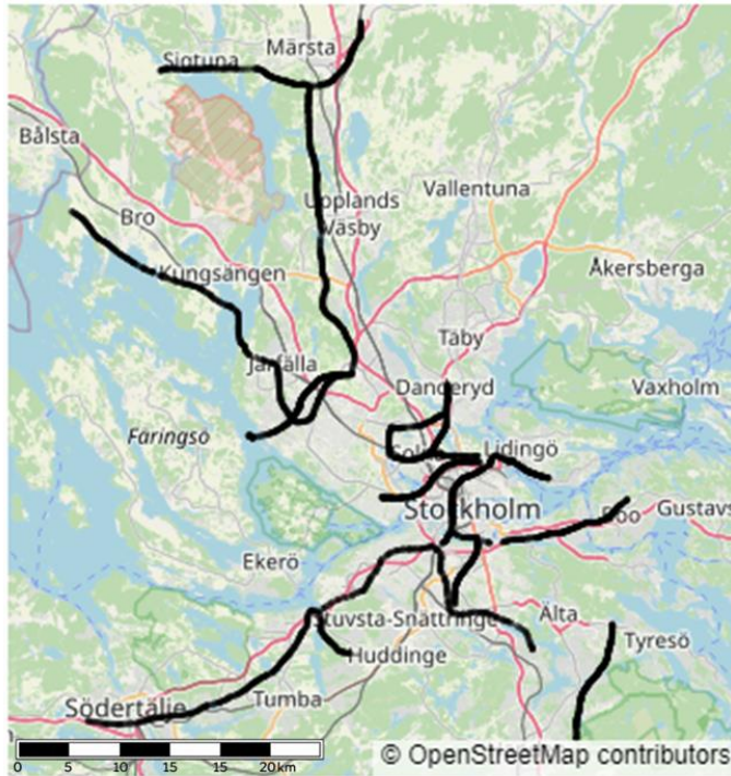
Figure 20: Approximate representation of the Stockholm DH network (DHN), showing the main transmission lines and network extensions across the Stockholm region [156].
