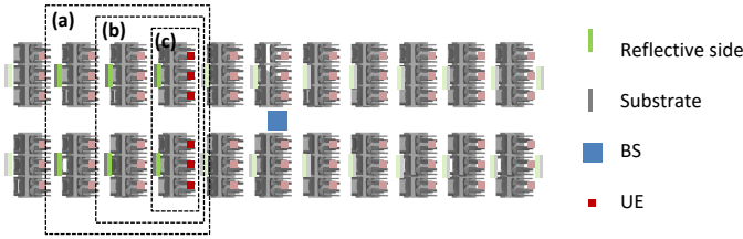
Figure 4.5.5: Illustration of different coverage group designs. Coverage group consists of (a) 6 ssRISs, 6 UEs; (b) 4 ssRISs, 6 UEs; (c) 2 ssRISs, 6 UEs.
