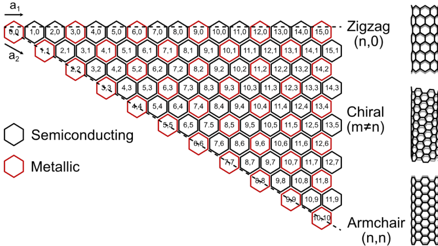
Figure 8: Chirality of carbon nanotubes. Integers inside the hexagons are n and m , describing the chiral vector
