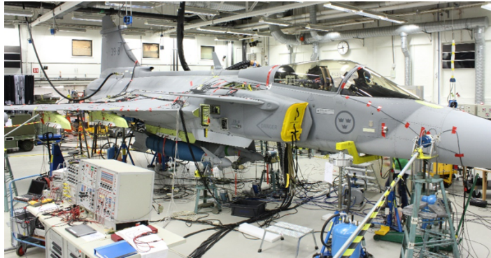
Figure 3.1.1: Ongoing ground vibration test of a JAS 39 Gripen E aircraft.
