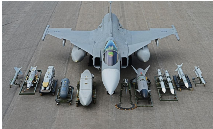
Figure 1.0.1: JAS 39 Gripen C with an assortment of external stores. Photo by Patrik Skolling Möller.
