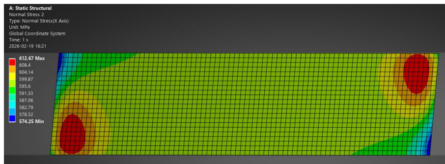
Figure 4-23: The normal stress surface profile of the specimen when the inner rollers are rotated 5 degrees
