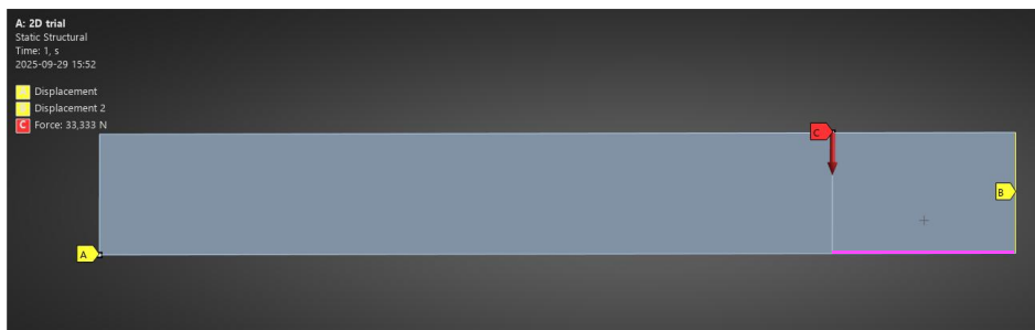
Figure 3-4: The boundary conditions of the model recreation, test surface is indicated via the pink line.
