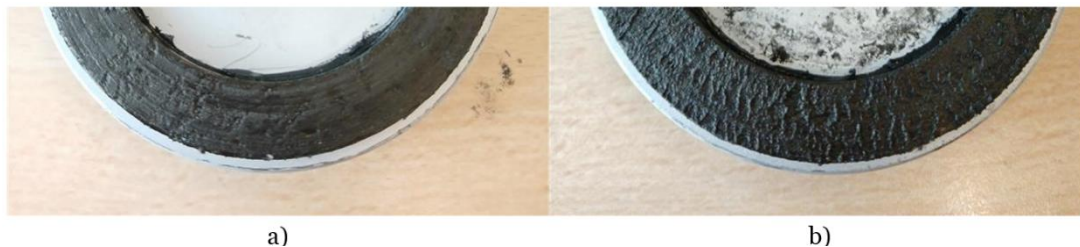
Figure 46. Facies comparison between a) 'one-way' mode and b) 'back and forth' mode at 90°C - Mix 1 - Ground A
