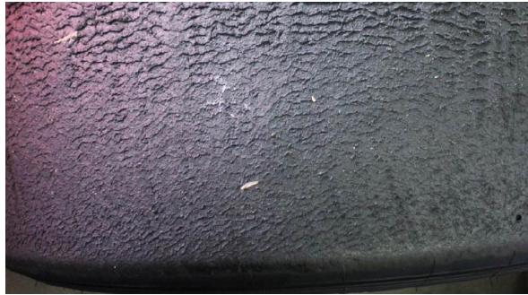
Figure 14. Photo of a tire tread showing graining [26]
