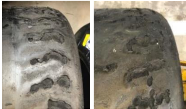
Figure 19. Example of blistering on the surface of a tire
