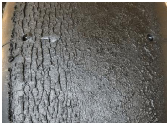
Figure 18. Example of graining on the surface of a tire
