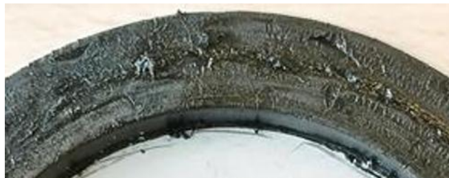
Figure 12. Sample with smearing on the surface
