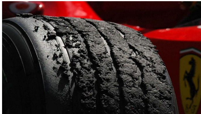
Figure 20. Tire with excessive pick-up [26]
