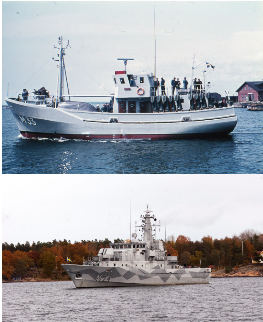
Figure 1.1.2: Early sandwich ships: HSwMS Viksten [10] (above) and HSwMS Kullen, a Koster-class ship [11] (below).
