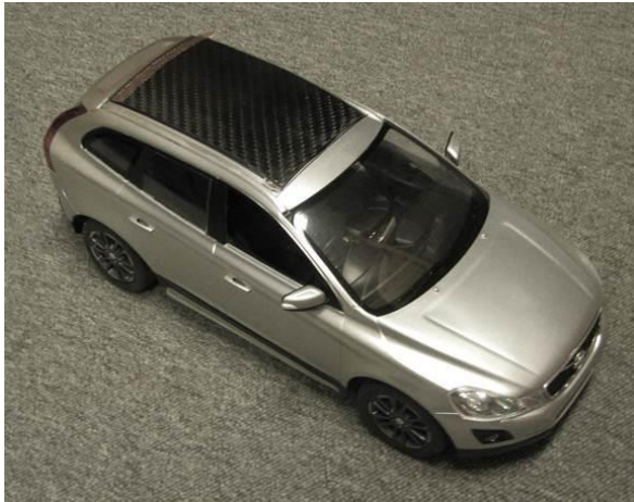
Figure 2. Model car showing the principle of a structural battery; the roof is replaced by a laminate super capacitor which is able to run the lights of the car. (Printed with permission from Swerea SICOMP AB).
