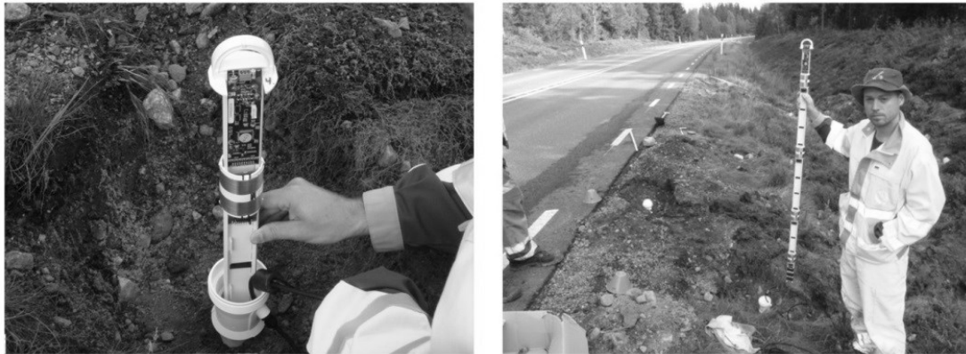
Figure 6. Capacitance moisture probe (left) and installation of a moisture rod in a test site in southern Sweden (photos from Klas Hansson).
