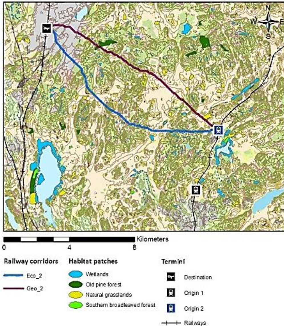
Figure 12. The results of the MCA-evaluation. The corridor with the highest overall score according to the three perspectives “ecology” (Eco_2), “geology” (Geo_2) and “neutral” (Eco_2). Elevation is represented by 4 m contours. Spatial habitat data previously published in (Mörtberg et al., 2012, 2007). Spatial data ©Lantmäteriet i2012/920.
